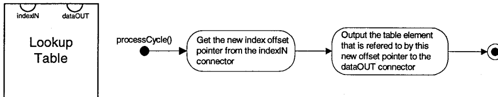
Figure 22: Schematic representation and activity diagram of the Lookup Table component.
