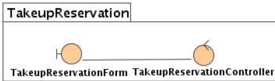
Figure 2.13: <<boundary>> and <<control>> Class for the Use Case Take Up Reservation
